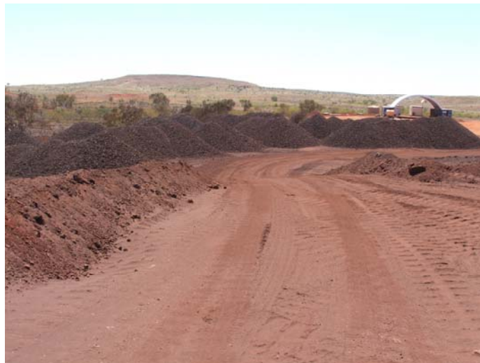
Photo: Ore yard at Ant Hill showing reprocessed and sampled ore piles ready for trucking to Port
