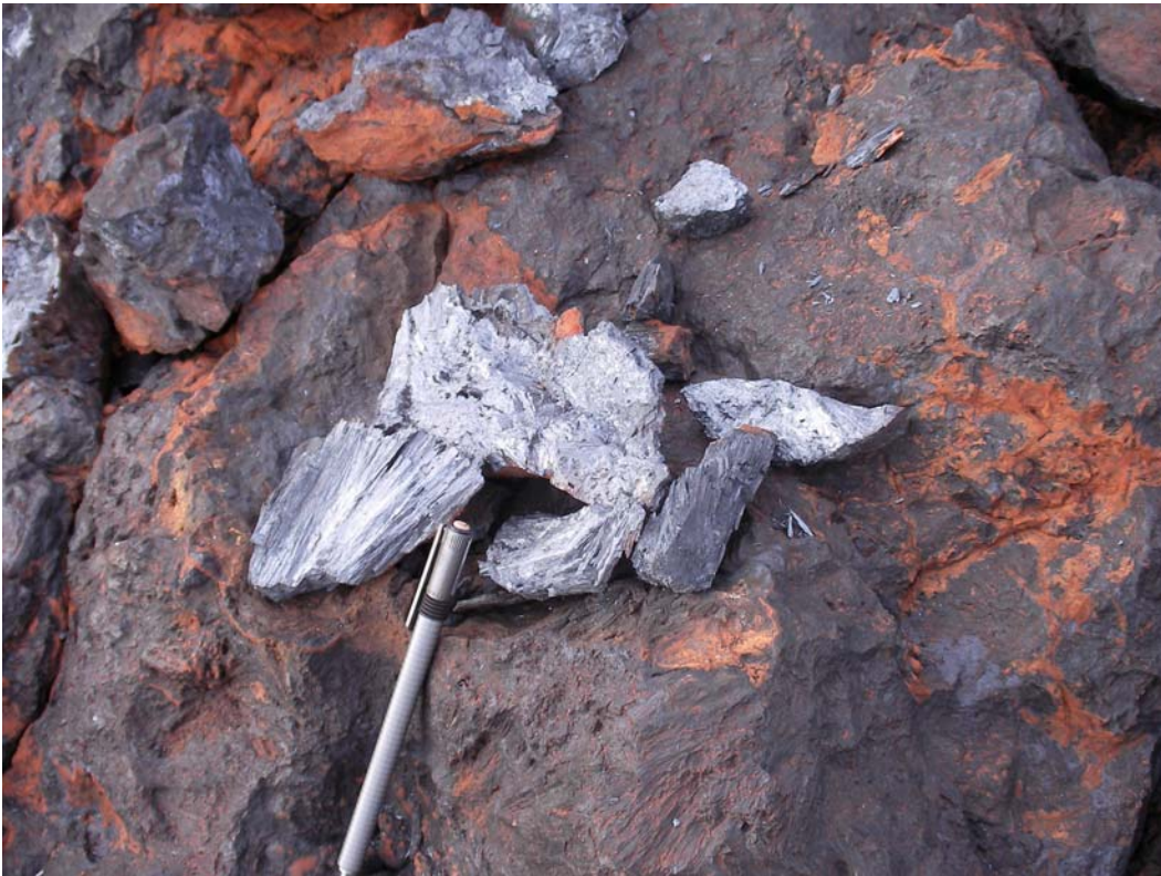
Typical crystal specimens of manganese oxide mineral from Sunday Hill outcrop. (Sample SHK00005 shown, which assayed: 59.60%Mn; 1.17%Fe; 0.59%Si; and 0.04%P)
